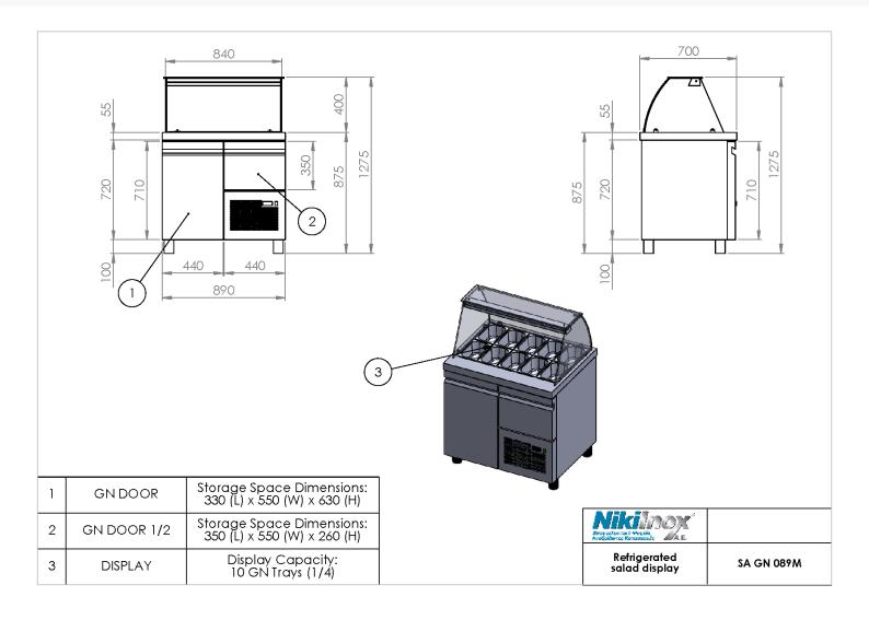
All refrigerators have insulation polyurethane, 1 shelf per door, magnetic sealing rubbers (Easy to change) and electronic thermostat with automatic defrost.
