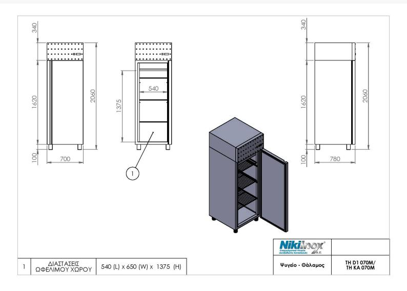
All refrigerators have insulation polyurethane, 3 shelf's per big door, magnetic sealing rubbers (easy to change) and electronic thermostat with automatic defrost.
